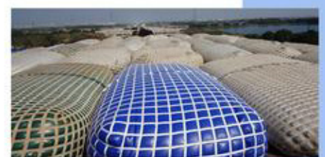
Bridge Preload Test
